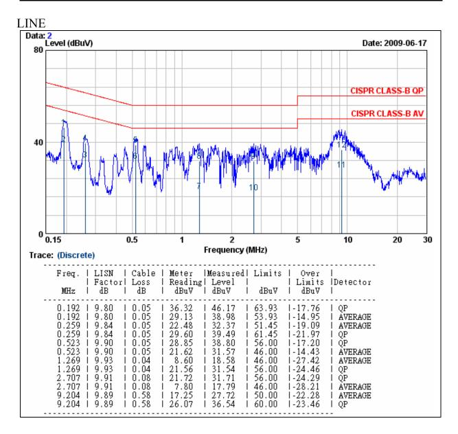
**REMARKS :** 1. Level (dBuV) = Read Level (dBuV) + LISN Factor (dB) + Cable Loss (dB) 2. Over Limit value (dB) = Level (dBuV) – Limit Line (dBuV)
