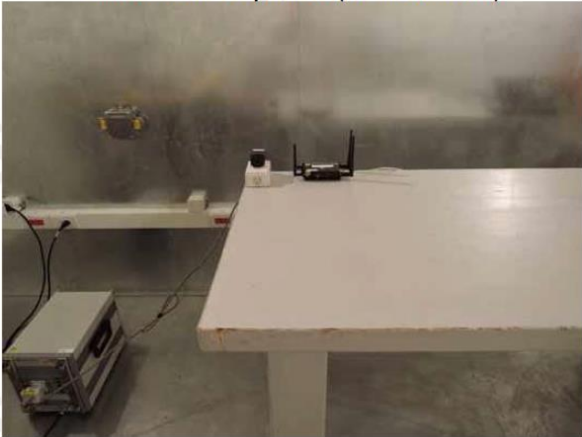
Conduction Setup Photo (AC Power Line)
