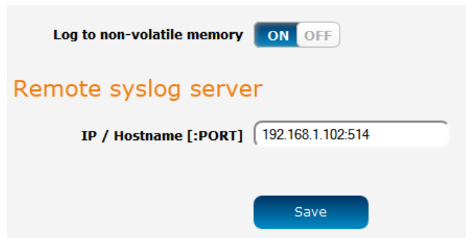
Figure 114 – Remote syslog server configuration
