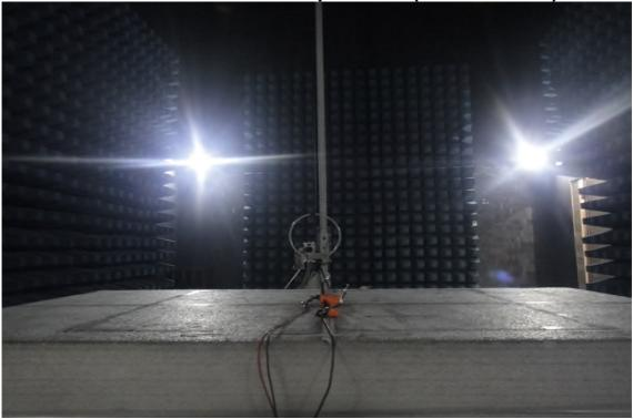
Radiated Emission Set up Photos (Below 1GHz)
