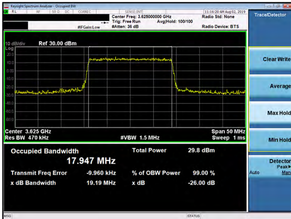
Plot 7-10. Occupied Bandwidth Plot (Band 48 - 20.0MHz QPSK - Full RB Configuration)
