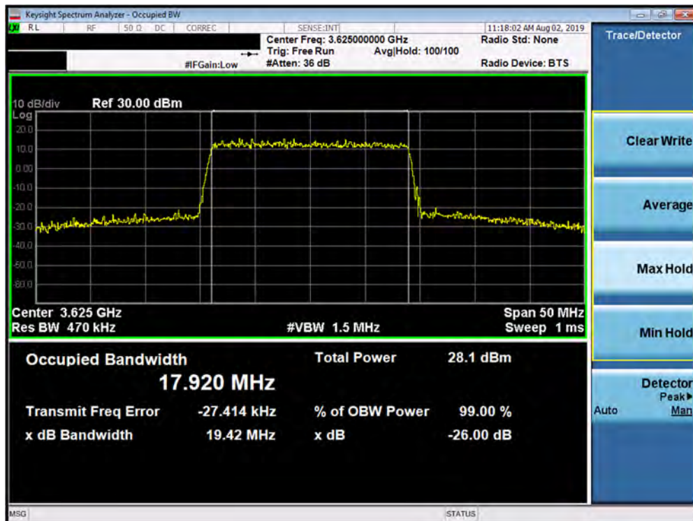
Plot 7-12. Occupied Bandwidth Plot (Band 48 - 20.0MHz 64-QAM - Full RB Configuration)
