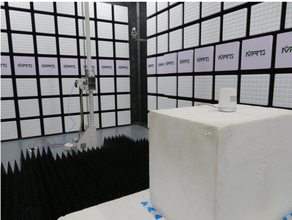
Description: Radiated Emission Test Setup Above 1GHz
