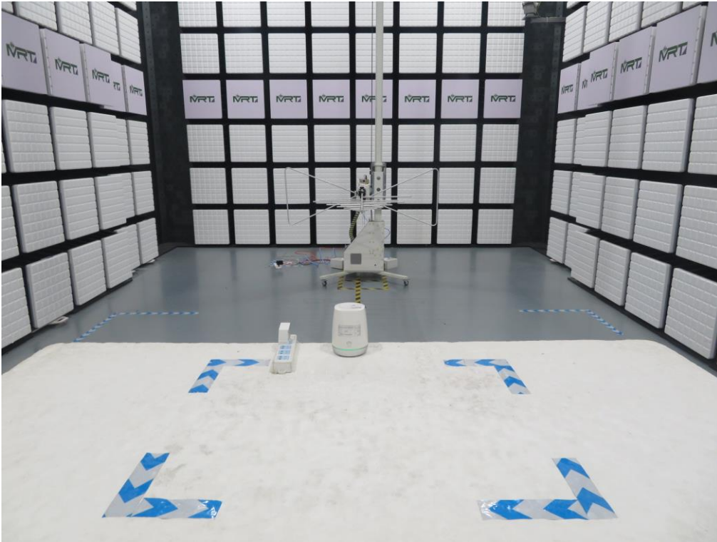
Description: Radiated Emission Test Setup Above 1GHz
