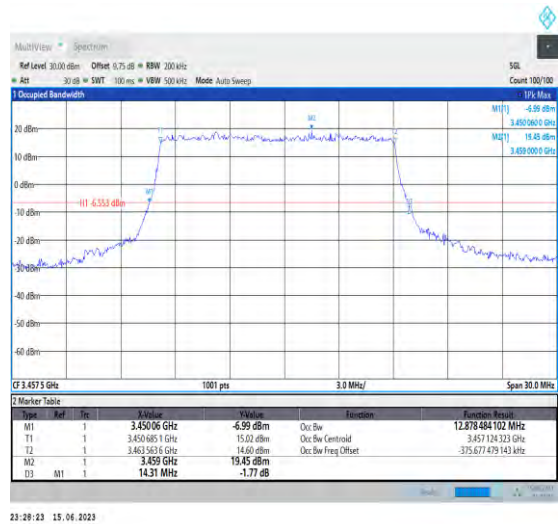
1-N78-3450-3550-PC1.5-30-15-L-1-DFT-QPSK-Outer er_Full-36@0-Ant1-12.878-14.310-≤15-PASS
