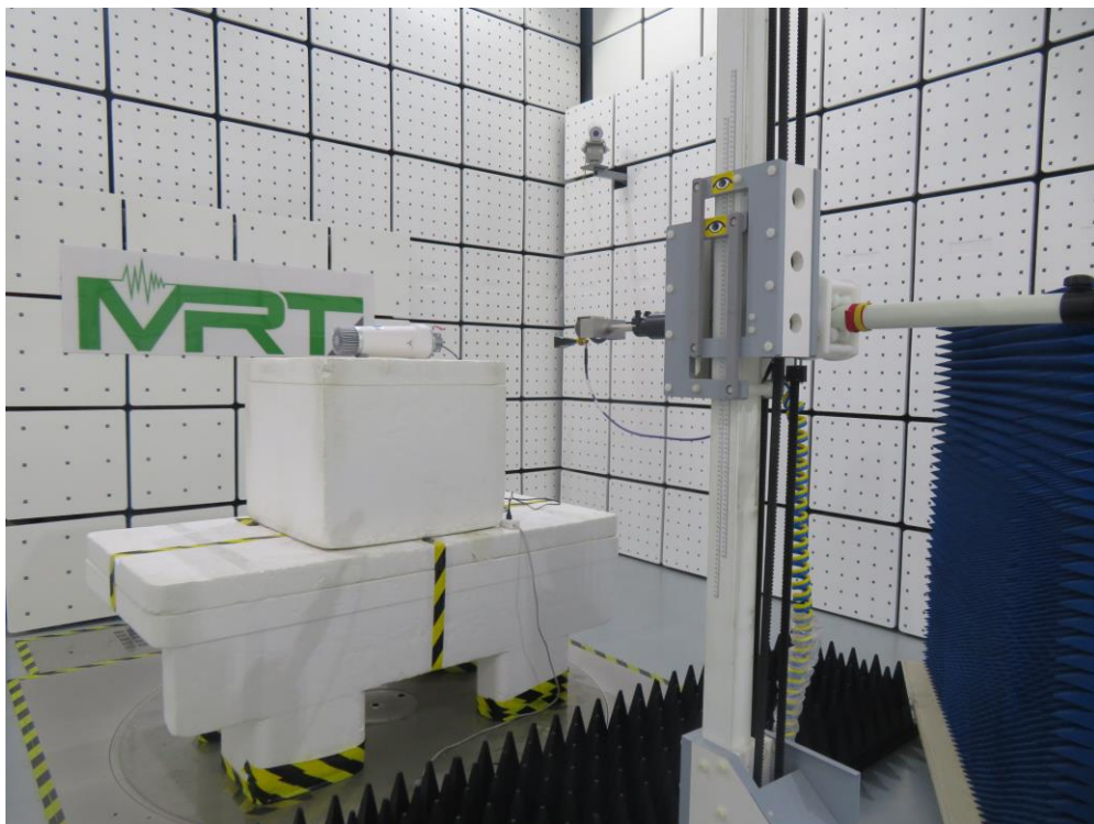
Description: Radiated Spurious Emission Test Setup for 40-50GHz
