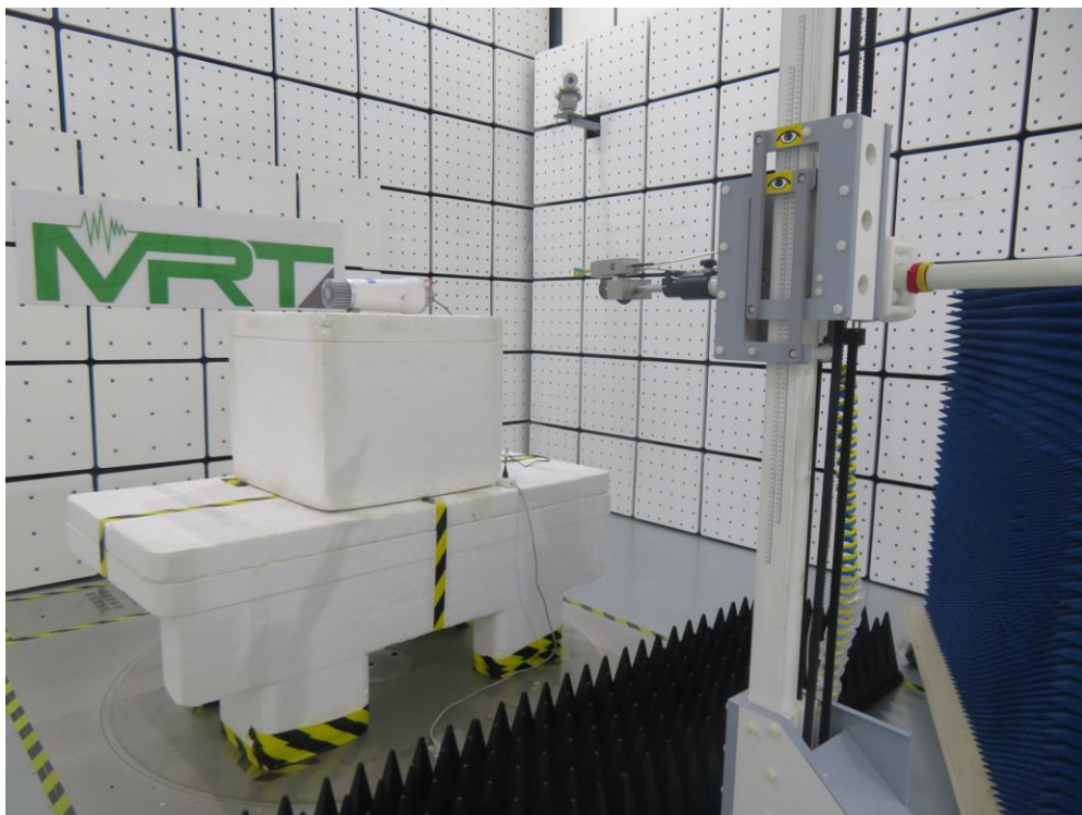
Description: Radiated Spurious Emission Test Setup for 75-100GHz
