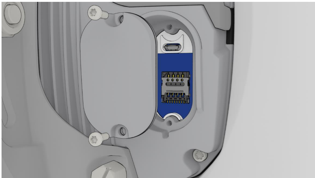
Figure 3 - Removing screws from the SIM hatch
