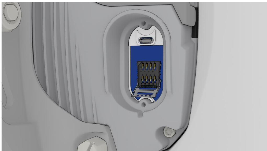
Figure 4 – Opening the SIM locking mechanism
