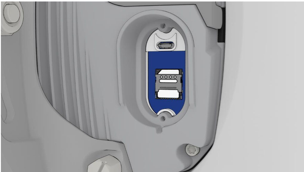
Figure 6 - SIM card locked in place
