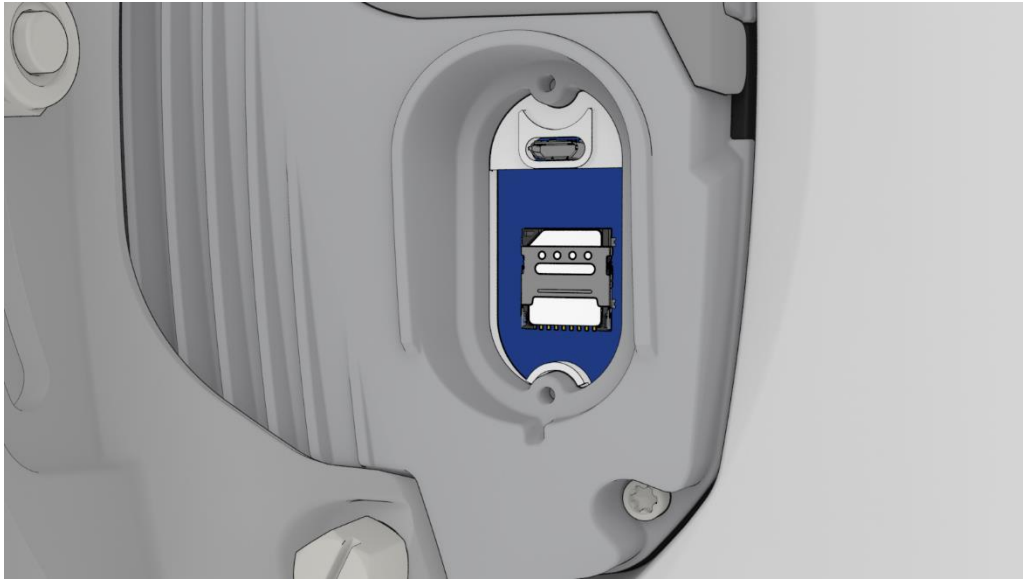
Figure 6 - Lock SIM card in place
