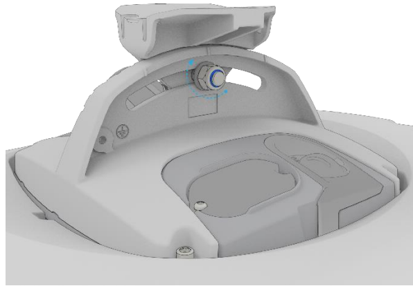
Figure 11 - Assembling pipe bracket to pole.
