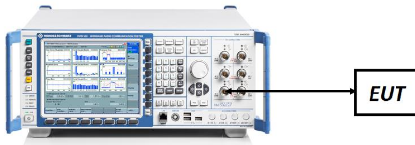
Figure 7-7. ERP/EIRP Measurement Setup
