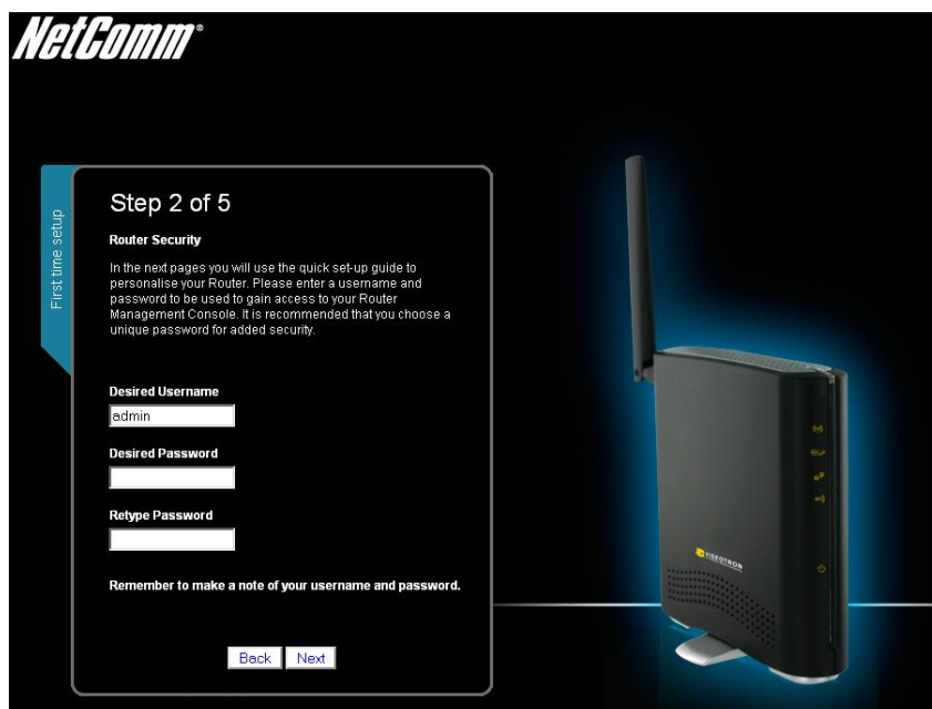
Figure 4 - Startup Wizard - Web Configuration Username and Password Settings
