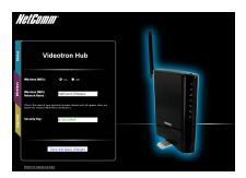
This page allows you to configure basic WiFi settings for this device such as enabling/disabling the WiFi functionality, changing the Wireless Network Name (SSID) and Wireless Security settings.
