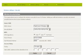
Your 3G36W-V uses WPA-PSK by default. Check your Wireless Security Card or device label on the bottom of the 3G36W-V for your default SSID and Security key to begin connecting your wireless devices.
