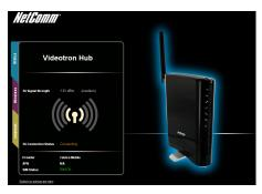
The status page shows the 3G connection status, Signal Strength (dBm) and SIM Status.
