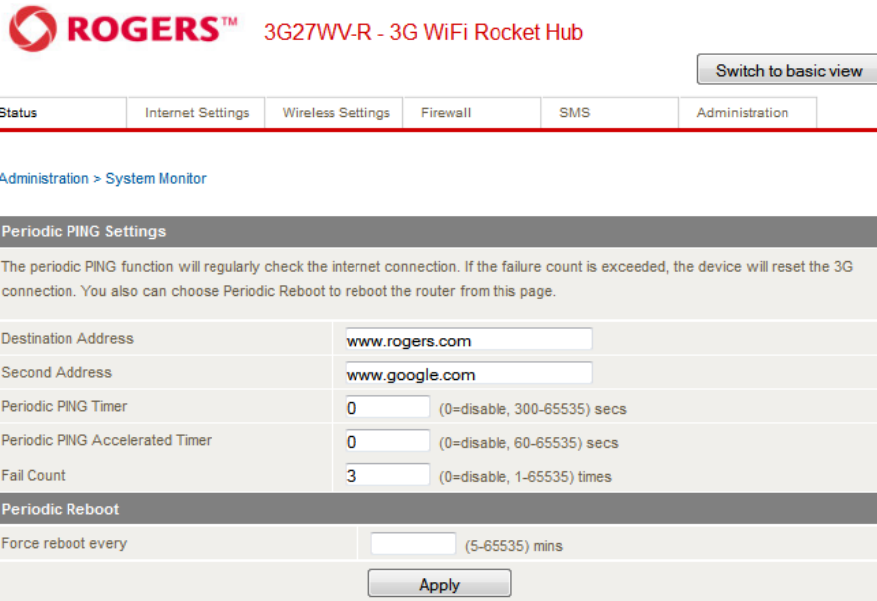
Figure 43 - Advanced View - System Monitor Settings
