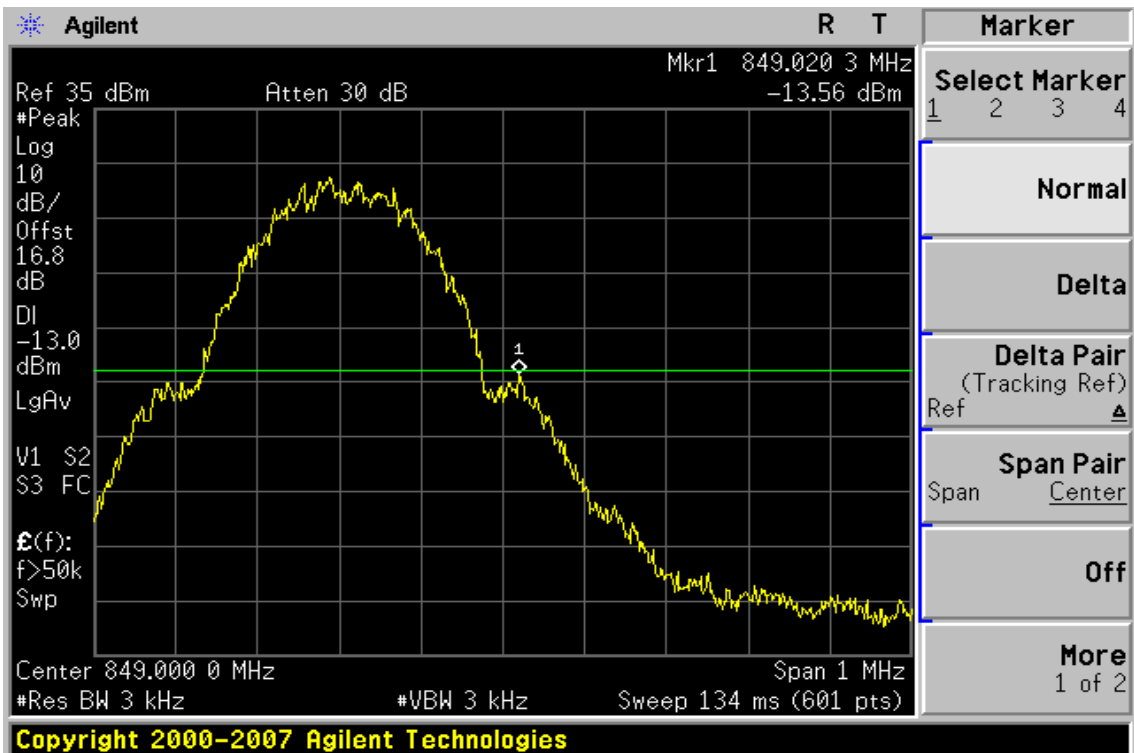
Figure 8-5: Band edge emission at antenna terminals – GSM 850 Channel Highest
