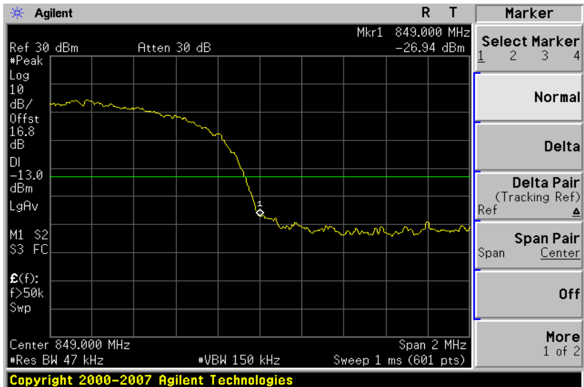
Figure 8-25: Band edge emission at antenna terminals –WCDMA V Channel Highest
