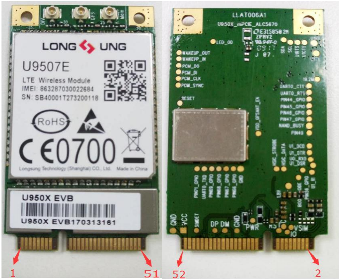
Figure 2-5 The Mini PCIe Interface pin sequence of U9507E
