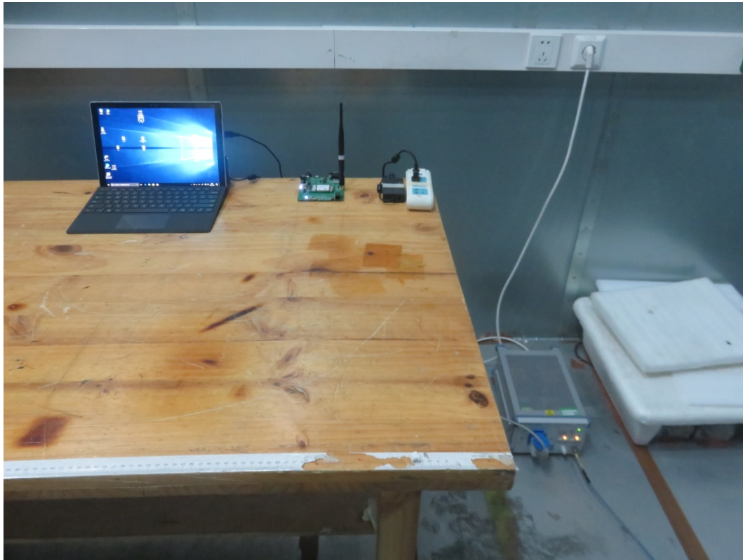
Picture 3 Conducted Emission Test Setup
