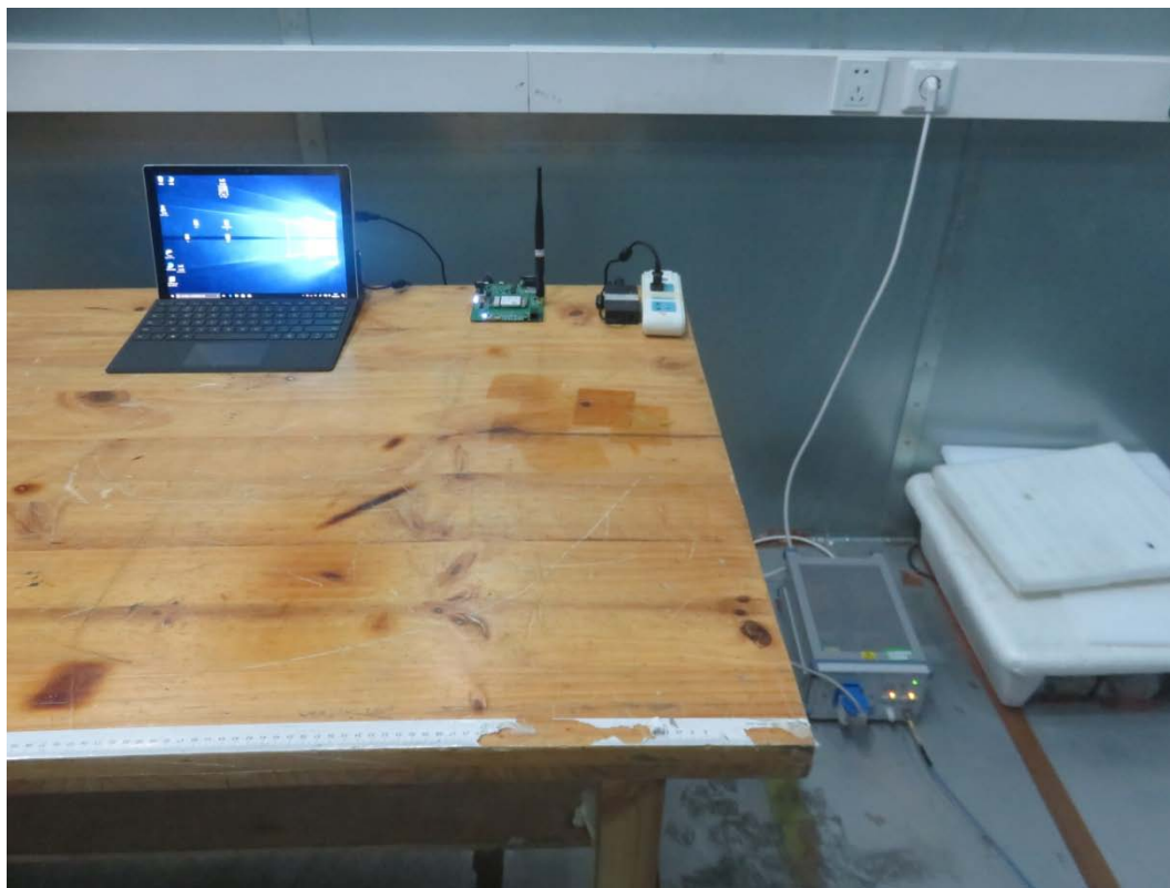
Picture 3 Conducted Emission Test Setup
