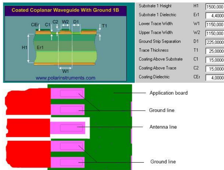
Figure 2-10 Micro-Stripline on 1.5mm standard FR4 2-layer PCB-example 2
