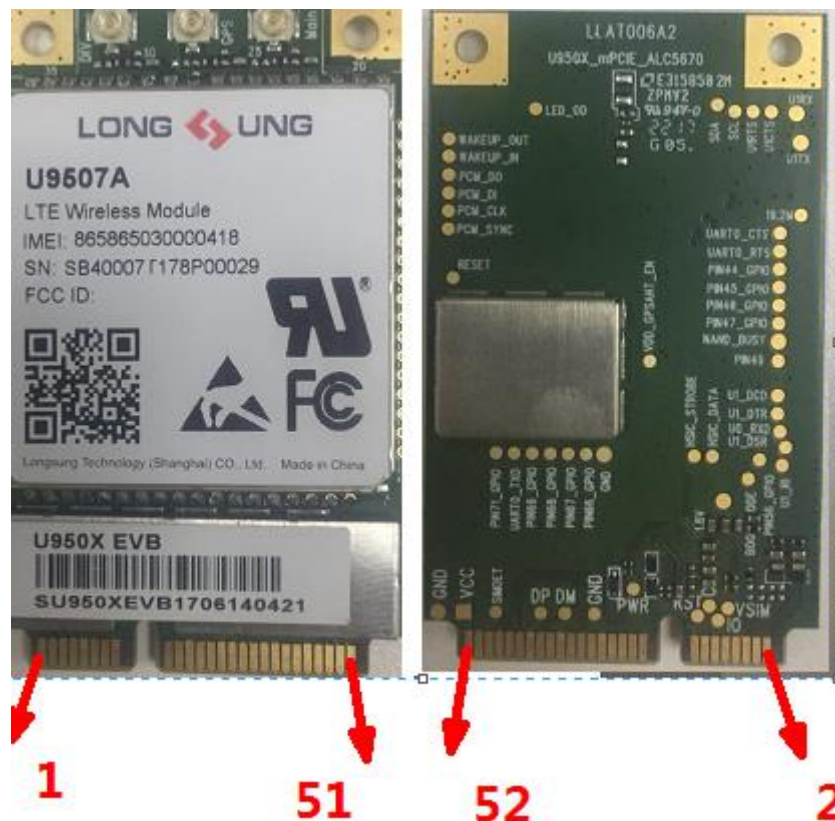
Figure 2-5 The Mini PCIe Interface pin sequence of U9507A
