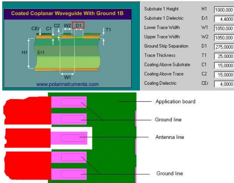
Figure 2-8 Micro-Stripline on 1.0mm standard FR4 2-layer PCB-example 2
