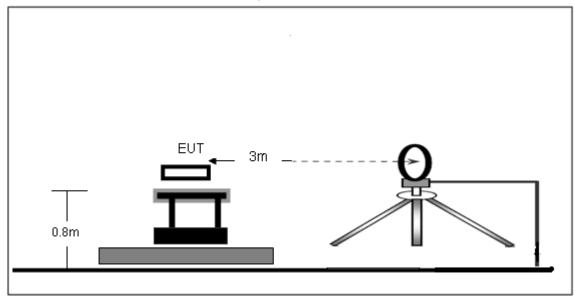
(B) Radiated Emission Test-Up Frequency 30MHz~1GHz
