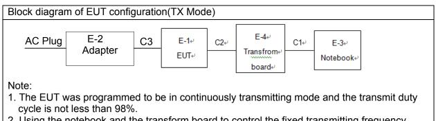
2. Using the notebook and the transform board to control the fixed transmitting frequency and other test mode. After finishing the test setting, the notebook and the transform board will be removed during measurements.
