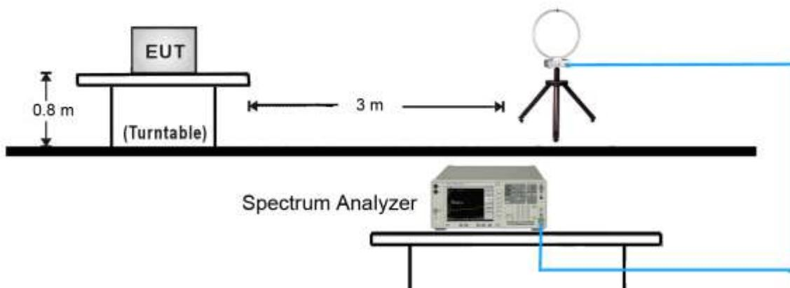
Below 1GHz Test Setup:
