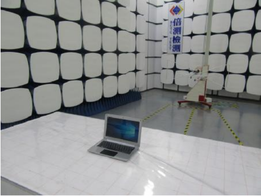
Radiated Measurement Photo
