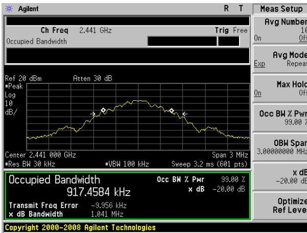
20dB Bandwidth plot on channel 78 (1Mbps)
