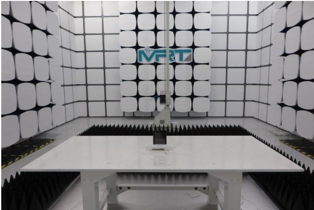
Description: Radiated Emission Test Setup for 18 ~ 25GHz
