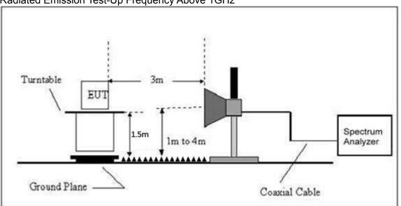
Radiated Emission Test-Up Frequency Above 1GHz
