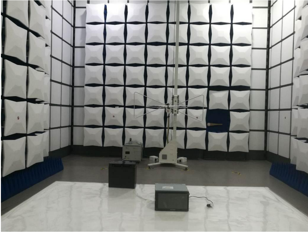
FCC RADIATED EMISSION TEST SETUP
