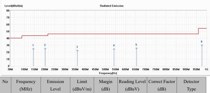
(dBuV/m) 1 143.870 24.55 43.50 -18.95 43.63 -19.08 QP \* 2 202.913 24.79 43.50 -18.71 46.39 -21.60 QP 3 361.768 22.13 46.00 -23.87 38.77 -16.64 QP 4 46.00 -21.66 36.78 QP 543.116 24.34 -12.44 5 654.174 25.44 46.00 -20.56 35.97 -10.53 QP 977.507 6 29.75 54.00 -24.25 35.75 -6.00 QP
