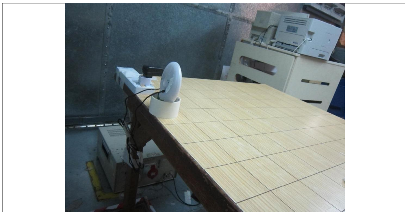
Conducted Emissions Test Setup (Rear View)
