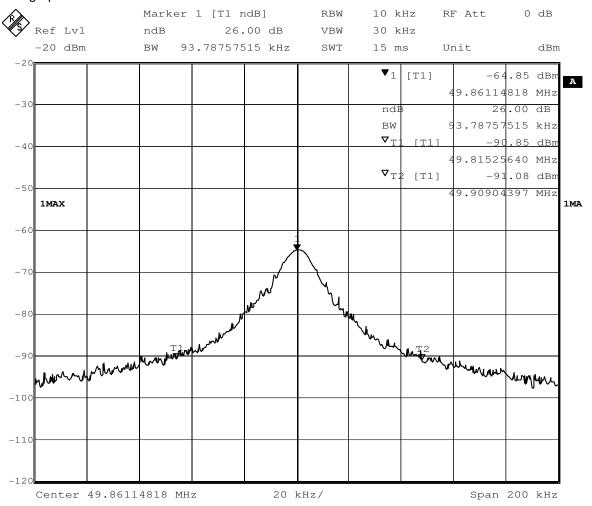
26dB bandwidth lower frequency :49.81525640MHz 26dB bandwidth upper frequency :49.90904397MHz
