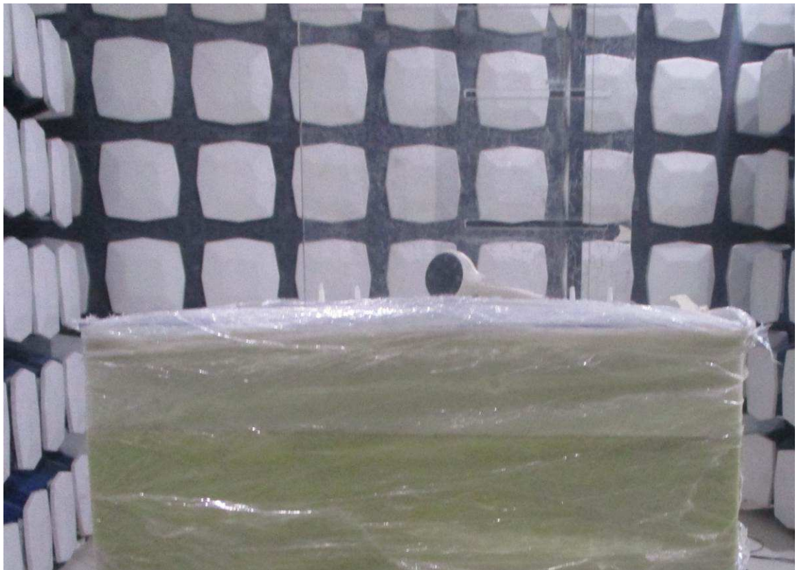
Above 1GHz (The EUT placed at the center of the turntable)
