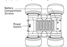
The remote control requires one 9V alkaline battery (not included). Loosen the screw using a phillips or cross screwdriver to remove the battery cover. Insert the battery according to the diagram inside the battery tray. Replace battery cover and tighten screw.
