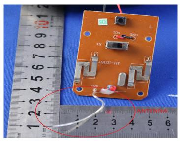
The antenna is integrated on the main PCB and no consideration of replacement. The best case gain of the antenna is 3dBi.
