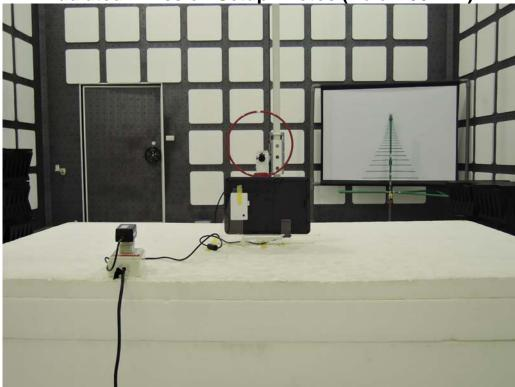
Radiated Emission Setup Photos (Below 1GHz)
