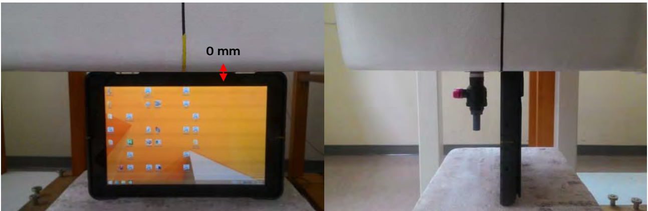
Fig.4 EUT Top side to flat phantom
