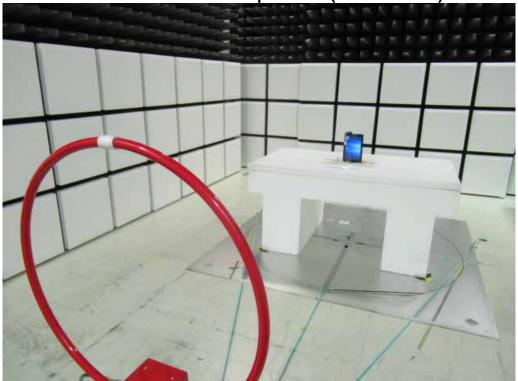
Radiated Emission Setup Photos (30MHz~1GHz)
