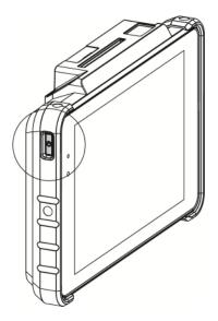
1. Push the power button to turn on the system and hold 4~5 seconds to turn off the system.
