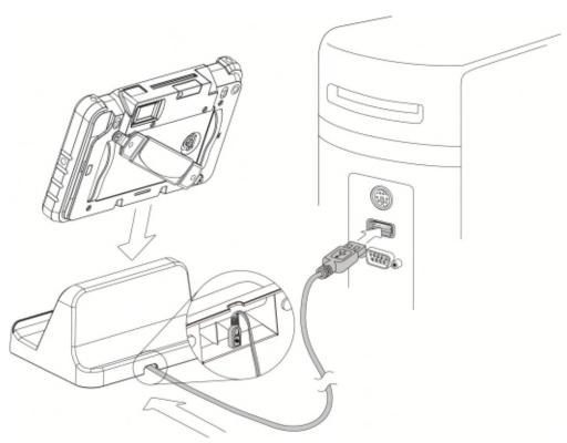
Connect the OTG USB cable to the connector on the bottom of the cradle charger and connect the other end to a PC to synchronize the two devices.
