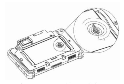
1. Loosen the pen screw counter-clockwise on the battery cover.
