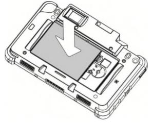
3. To install the battery put the battery in the slot and push until the battery clicks into place.
