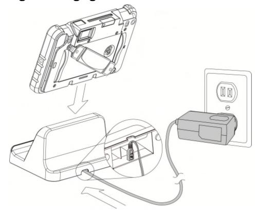
1. Connect the USB-AC adapter to the connector on the bottom of the cradle charger and the power outlet.
