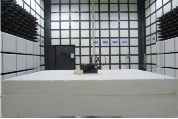
Radiated Emission Setup Photos (Below 1GHz)
