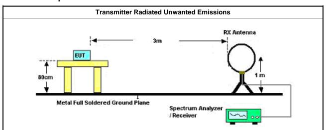
Magnetic field tests shall be performed in the frequency range of 9 kHz to 30 MHz using a calibrated loop antenna. The center of the loop shall be 1 m above the ground.
