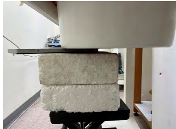
Fig.3 EUT Back side to flat phantom
