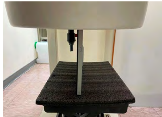
Fig.4 EUT Top side to flat phantom
