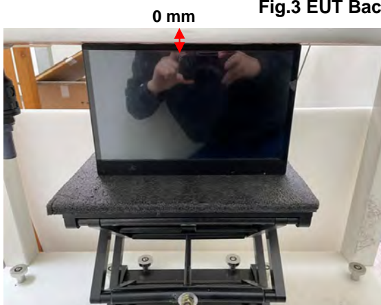
Fig.4 EUT Top side to flat phantom
