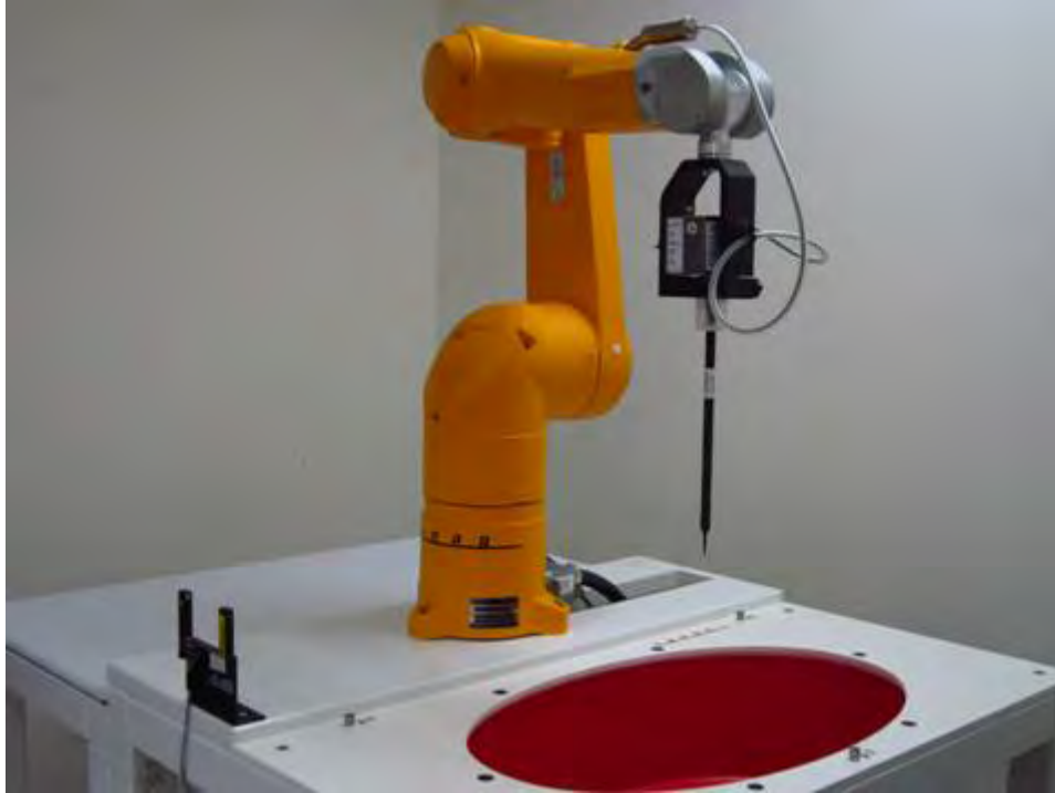
Fig.1 Photograph of the SAR measurement system
