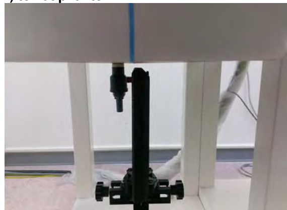
Fig.8 EUT Left side (10mm) to flat phantom
