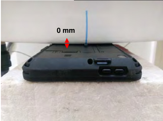
Fig.3 EUT Back side (Main) to flat phantom
