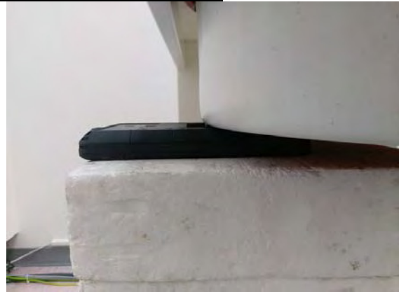
Fig.3 EUT Back side (Main) to flat phantom
