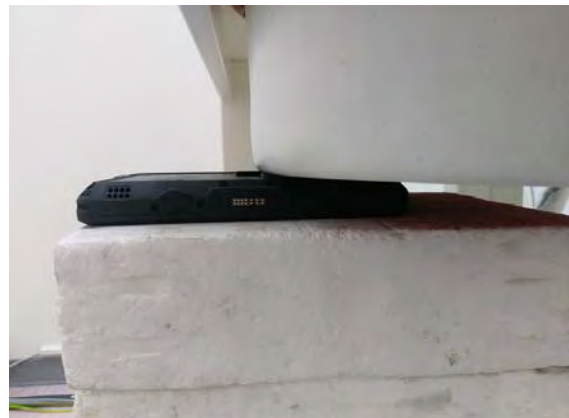
Fig.4 EUT Back side (Aux) to flat phantom
