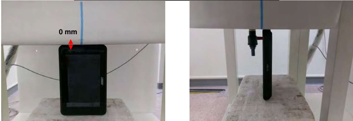
Fig.9 EUT Right side to flat phantom
