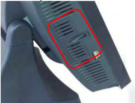
HDD access panel
