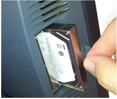
The HDD/SSD may be hot swapped when in a RAID 1 configuration. In non-RAID 1 configurations the unit should be powered down before changing a drive or data may be lost. No physical damage will happen to the HDD if inserted or removed with power on.
