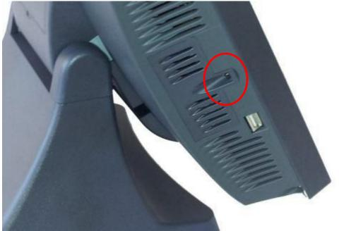
Remove or insert drive as needed
