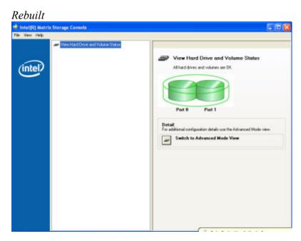
The RAID has now mirrored the drive and the system is now protected for a drive failure.
