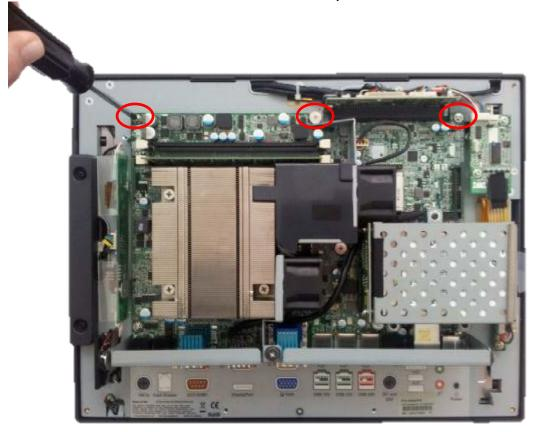
After the screws are removed the system board can be unplugged from its connector. While using the I/O bracket to pull on, slide the board out towards the bottom of the unit as shown.
