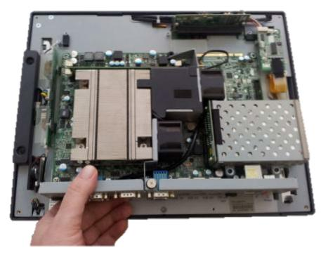
When reinstalling the system board make sure the locking tabs on the bottom of the board lock into their mating slots.
