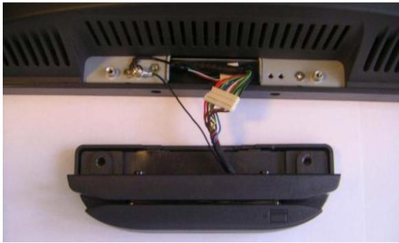
Attach the MSR using the two screws at the locations shown below.
