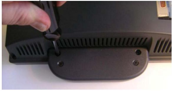
Connect the cable together as shown add secure the static ground wire with screw provided as shown.
