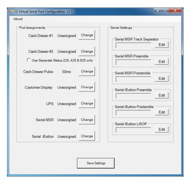
Virtual serial ports can be used for the cash drawers, virtual 2x20 line display on the optional 10.1 LCD, Smart UPS, MSR and iButton.
