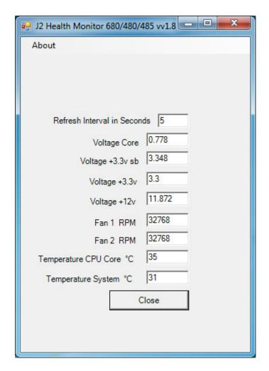
As can be seen above, when running on the J2 680 the J2 Health program displays critical system voltages and system and CPU Core temperatures. For other J2 POS systems, J2 Health may display more or less information. An example would be the J2 680 unit, which in addition to the above information would also display the fan speed of the two J2 680 fans.
