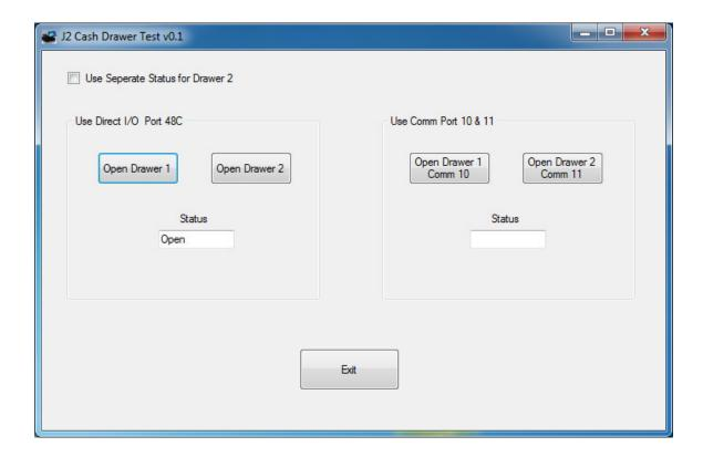
The "Use Comm Port 10 & 11" option is to test the cash drawer you set up using the J2 virtual serial ports program. The virtual serial port program must be installed with the cash drawer virtual serial ports set to Comm 10 & 11.
