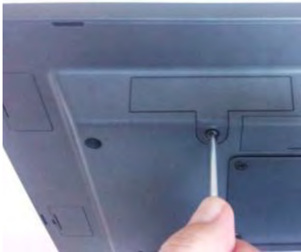
HDD access panel
