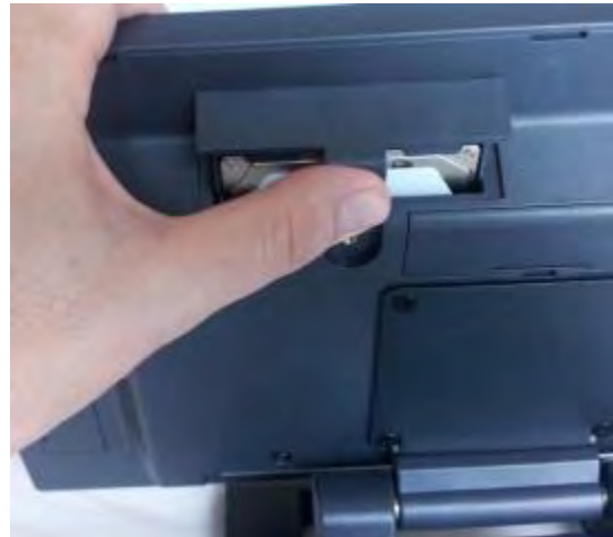
HDD slide in-slide out drive bay
