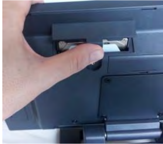
HDD slide in-slide out drive bay
