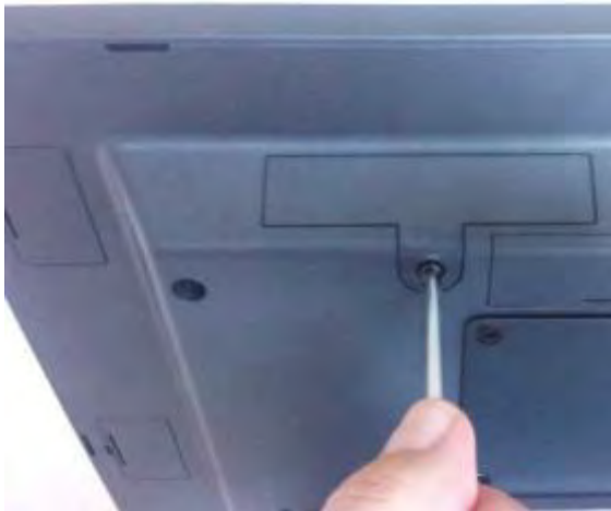
HDD access panel
