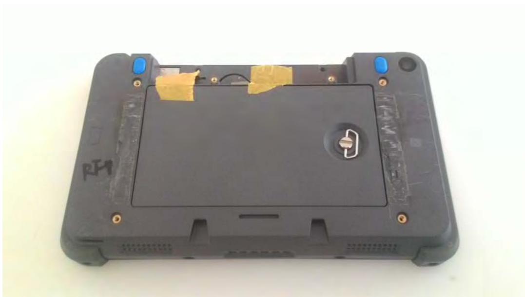
Fig.10 Back view of EUT (remove scanner and rails for SAR testing via KDB inquiry)
