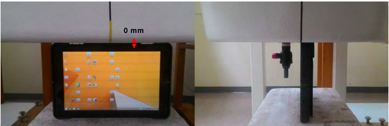
Fig.4 EUT Top side to flat phantom
