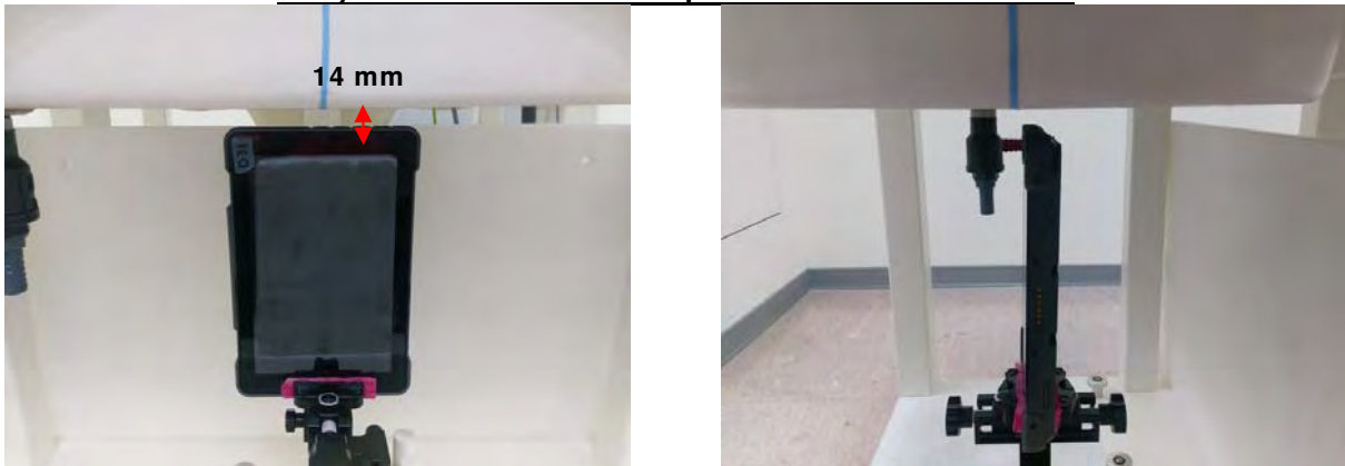
Fig.7 EUT Top side to flat phantom
