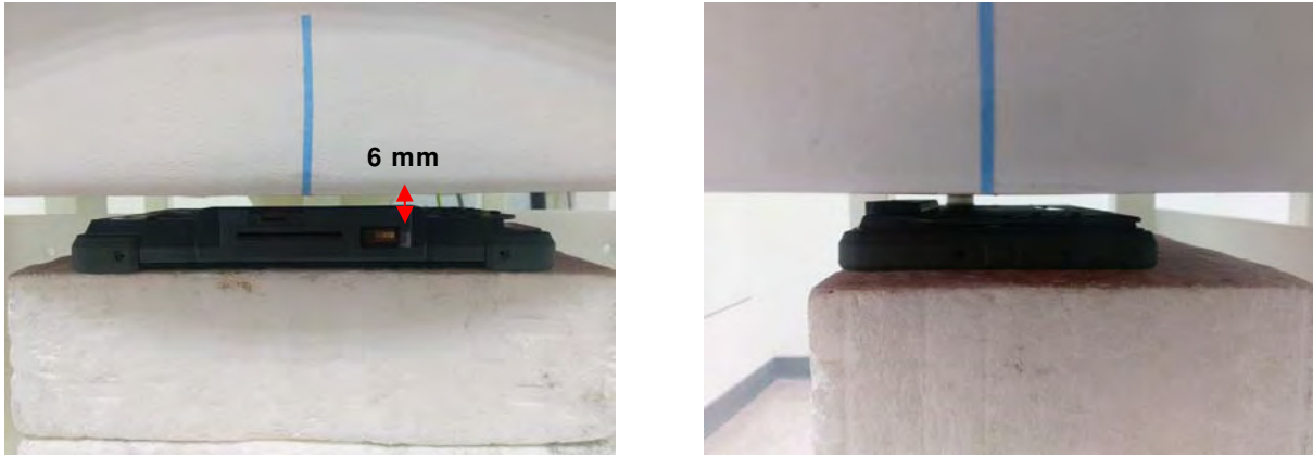
Fig.6 EUT back side to flat phantom
