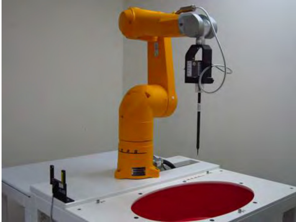
Fig.1 Photograph of the SAR measurement system
