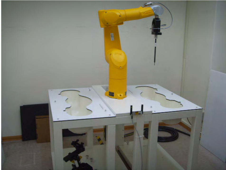
Fig.1 Photograph of the SAR measurement system
