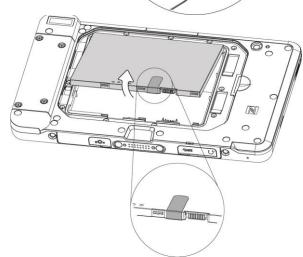
To install the battery cover, angle the battery cover so that the left side is inserted first into the battery compartment. Then press into place and slide the latch downward to lock the battery cover.
