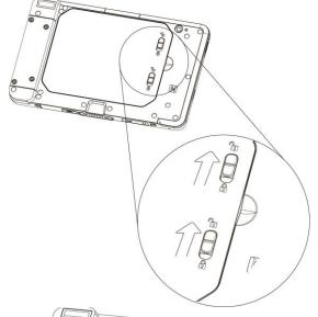
A plastic tab is attached to the battery module. For easier removal pull the plastic tab upwards to release the battery from the unit.
