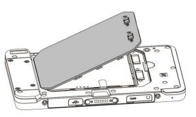
**Note:** When closing the battery cover, follow the number shown in the picture to press the cover until it snaps into place.
